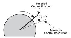
Actuator responds to a 175 mV signal when reversing direction from stop position.
