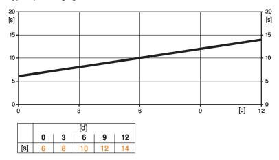
[d] = Power failure in days [s] = Pre-charging time in seconds
