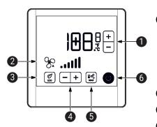
1 Temperature setpoint: Set the desired temperature
