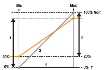
Nominal value (OEM setting) Nom Adjustment range Min 1 Adjustment range Max 2 Feedback U 0...100% Nom 3 Control Y Min...Max 4
