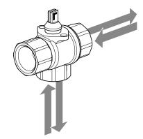
Delivery condition conforms to valve position 90°/positioning signal 10 V.
