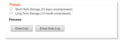
The data recording memory is a ring buffer. When it is full, the oldest element is replaced by a new one. The time stamp for the data recording is always in UTC.
