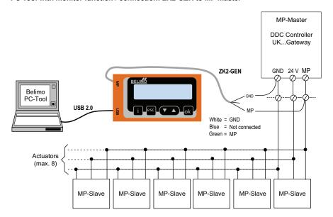
PC-Tool with monitor function / connection: tool socket with ZK6-GEN, ZK4-GEN
