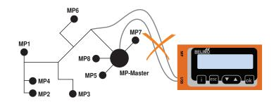
Solution: Use the service socket on the actuator or temporarily disconnect the MP connection of the MP device from the MP-Bus and connect the ZTH AP to the MP connection.
