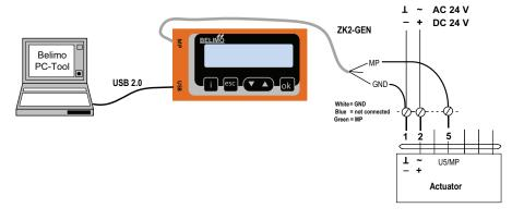
Note The USB driver required will be automatically installed with PC-Tool version 3.9 or higher. For older versions of the PC-Tool, the driver can be downloaded from www.belimo.com and installed separately.
