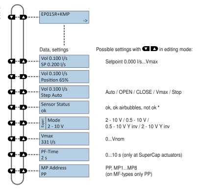
\* ok: Flow sensor is working properly ok airbubbles: Flow sensor is working properly, airbubbles in the system not ok: Sensor error
