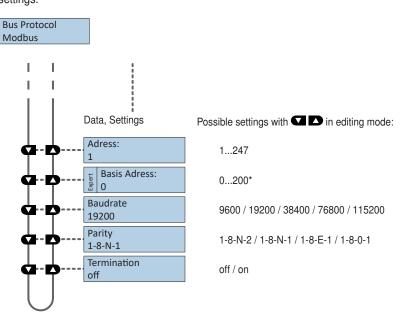
\*) The setting of the base address is also taken into account for the BACnet MS / TP address.
