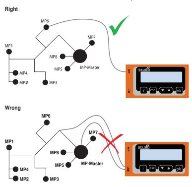
Solution: Use the service socket on the actuator or temporarily disconnect the MP connection of the MP device from the MP-Bus and connect the ZTH AP to the MP connection.
