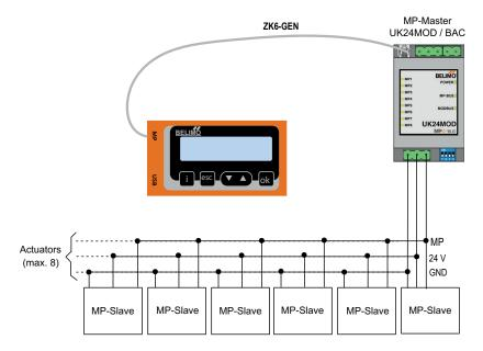
When the ZTH AP is connected to the Belimo actuator, the operating device starts and data is
