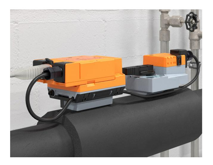
The Belimo Energy Valve and Thermal Energy Meter provide energy control and efficient energy billing. They offer an accurate measurement and monitoring of energy consumption in a heating and cooling system with direct IoT-based cost accounting using a single device. Designed to EN1434/CSA C900 standards, they ensure high accuracy and reliability, allowing for transparent tenant billing.
